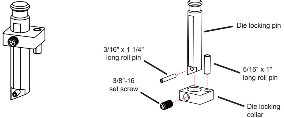
The purpose of the die locking pin, as its name suggests, is to lock the forming die in a set position to prevent the tubing from springing back. This is critical for bending thin wall tubing to help prevent wrinkling and also very strong, heavy wall tubing to limit spring back.
