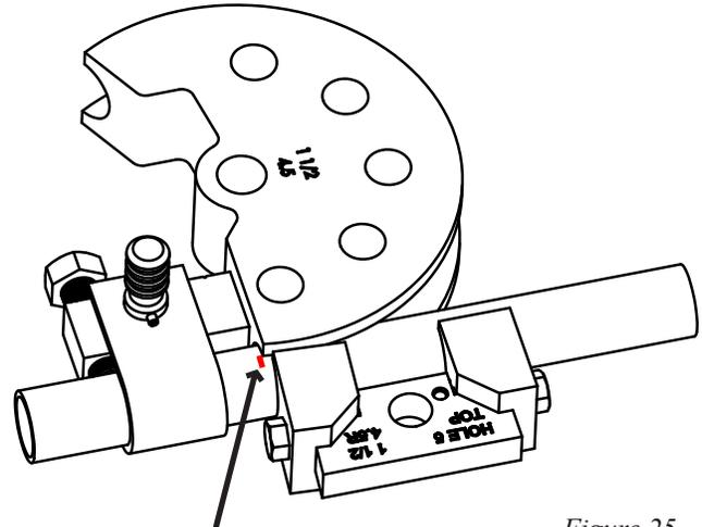
Mark here at the saw cut edge of die (not at the followbar's insert)
