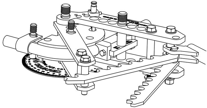
Figure 13 - Bending with drive holes and ratchet
