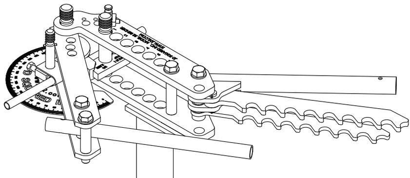
Figure 14 - Handle installed and ready to bend without drive holes
