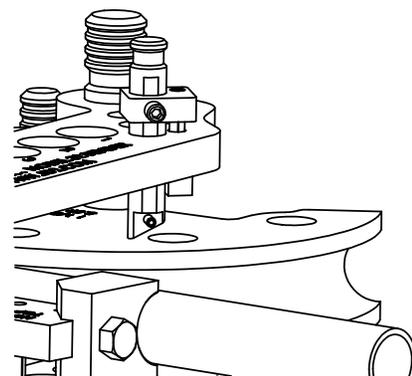
Figure 15 - Sliding along die's upper surface
