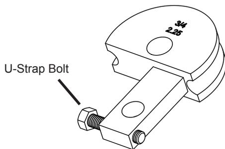
Figure 6 - Forming Die without drive holes
