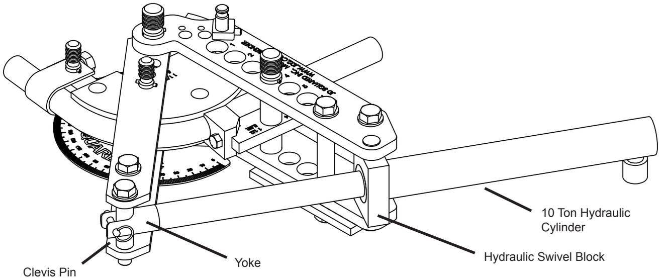
Figure 5 - Bender with hydraulics installed.
